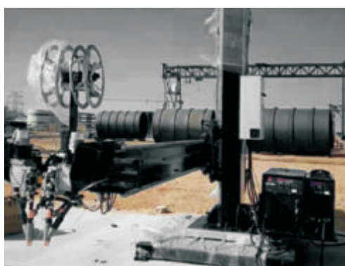
Longitudinal seam welding by manipulator
